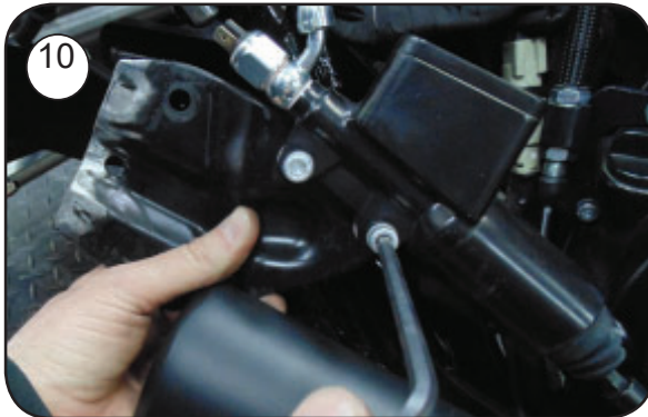
10. Attach master cylinder to modified exhaust bracket. Bolt old (modified) exhaust bracket to frame between new exhaust bracket and frame.
